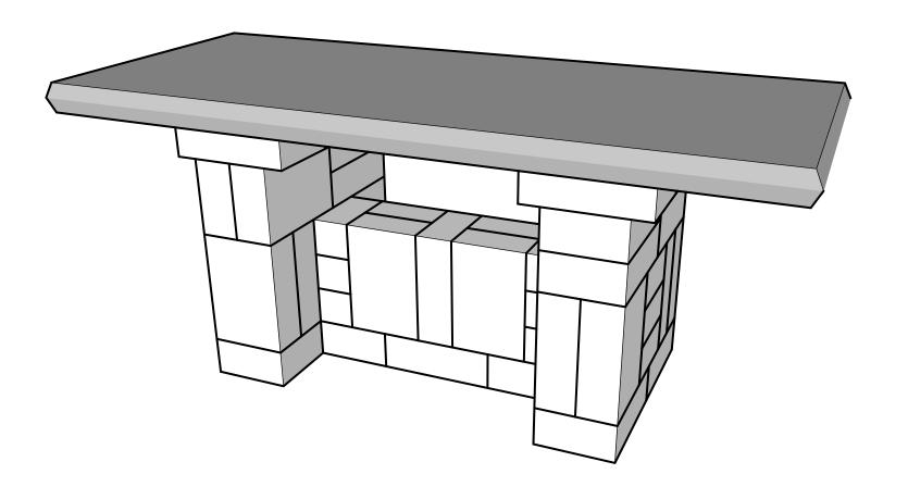
When constructing your project, be sure to keep all blocks level, square, and plumb. Use a four foot level and check often. Starting on a level foundation is key. When gluing blocks together, be sure not to use too much adhesive - this will cause the blocks to "swim." A small bead is ideal.
