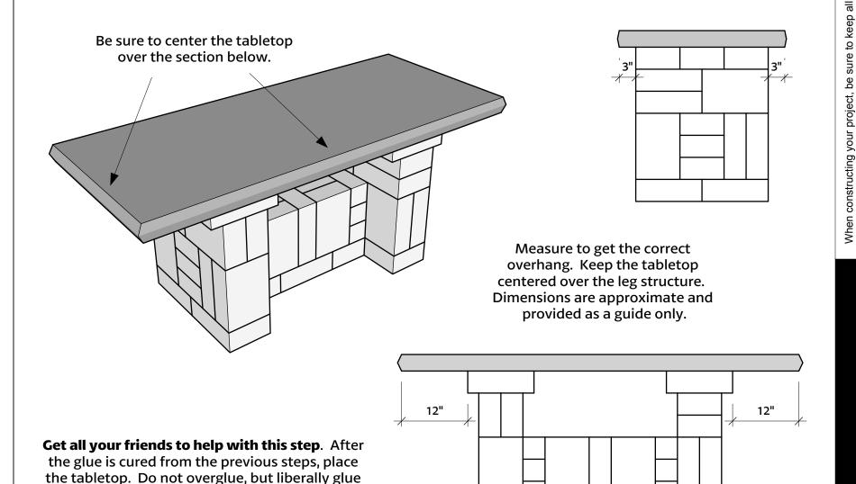
the block before placing the top. Do not glue too close to the blocks' edges. You will need "wiggle room" to center the tabletop.
