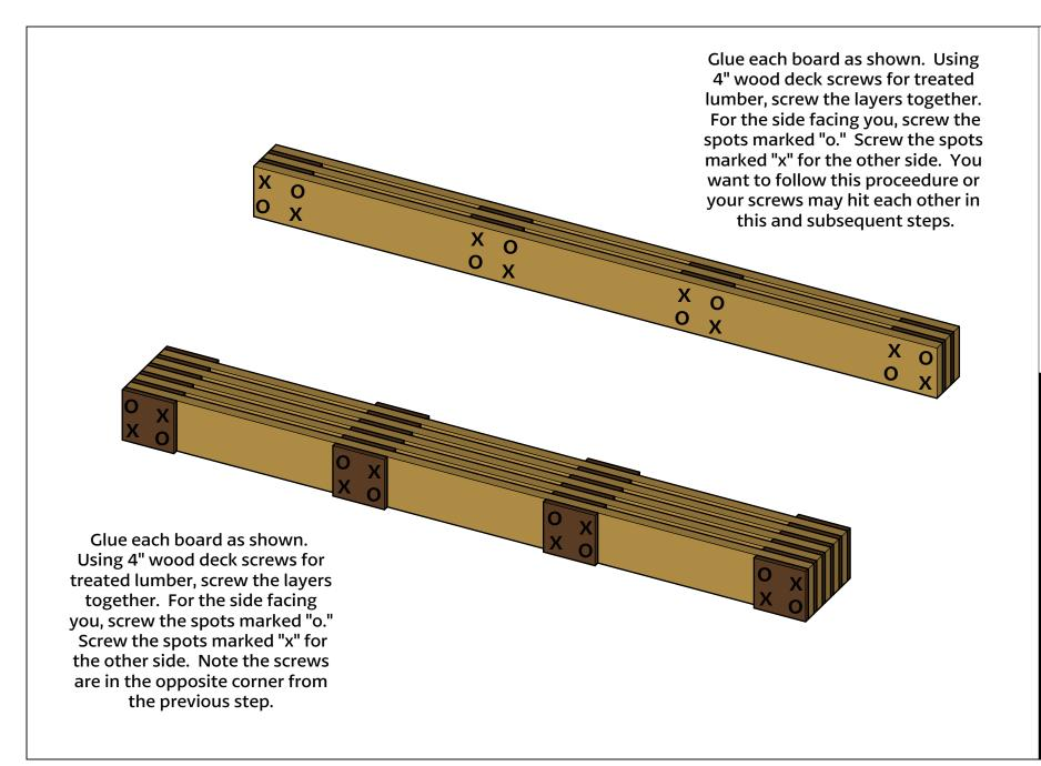
When constructing your project, be sure to keep all blocks level, square, and plumb. Use a four foot level and check often. Starting on a level foundation is key. When gluing blocks together, be sure not to use too much adhesive - this will cause
