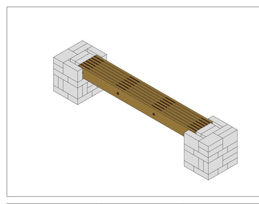
When constructing your project, be sure to keep all blocks level, square, and plumb. Use a four foot level and check often. Starting on a level foundation is key. When gluing blocks together, be sure not to use too much adhesive - this will cause the blocks to "swim." A small bead is ideal.
