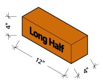
Long Halves are simply made by cutting a block along its center on the longest axis.
