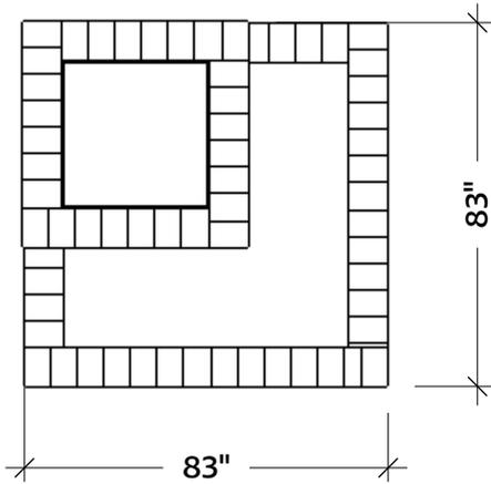
Any time you see a block with just the wide top showing, fret not, it is a Square Foot Unit (SFU). The unit is just turned where the that is the only block you see.
