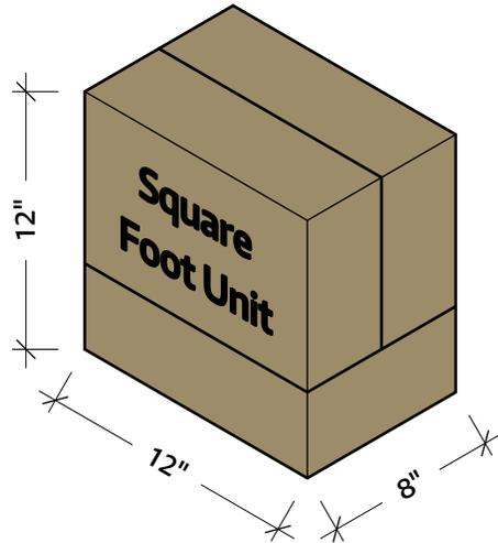
The "Square Foot Unit." consists of three blocks as shown. By rotating this unit (SFU) we are able to build quickly and easily while keeping bond lines broken up. These will always be shown in a tan color.
