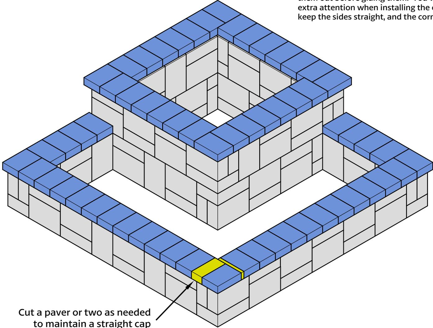
Cut a paver or two as needed to maintain a straight cap with proper overhang.
