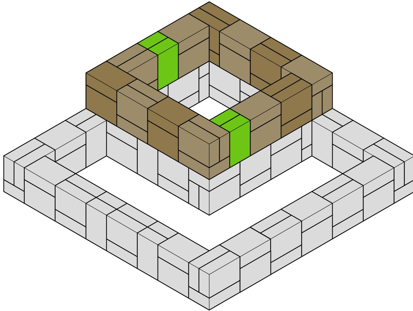
When constructing your project, be sure to keep all blocks level, square, and plumb. Use a four foot level and check often. Starting on a level foundation is key. When gluing blocks together, be sure not to use too much adhesive - this will cause the blocks to "swim." A small bead is ideal.
